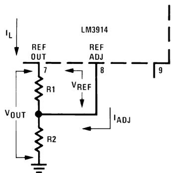
Since the 120 $\mu$ A current (max) from the adjust terminal represents an error term, the reference was designed to minimize changes of this current with  $V^+$  and load changes.
