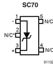
\*This pin must be left floating or connected to pin 1.
