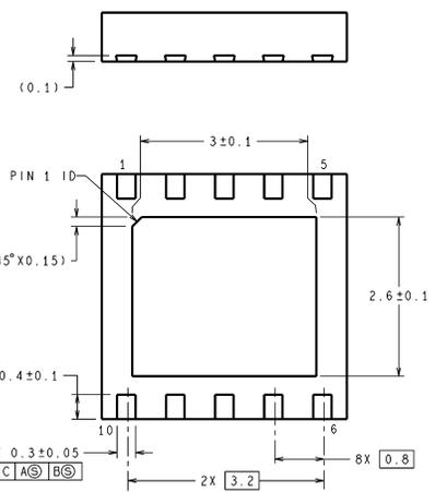
DIMENSIONS ARE IN MILLIMETERS
