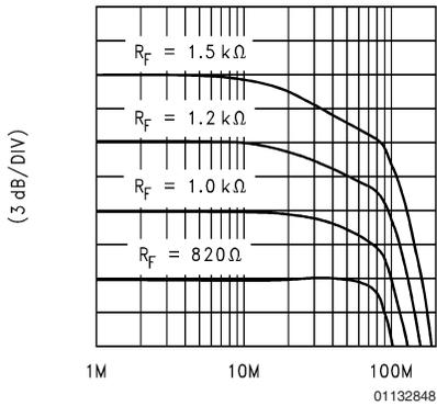
**BANDWIDTH vs  $R_f$  &  $R_S$**
