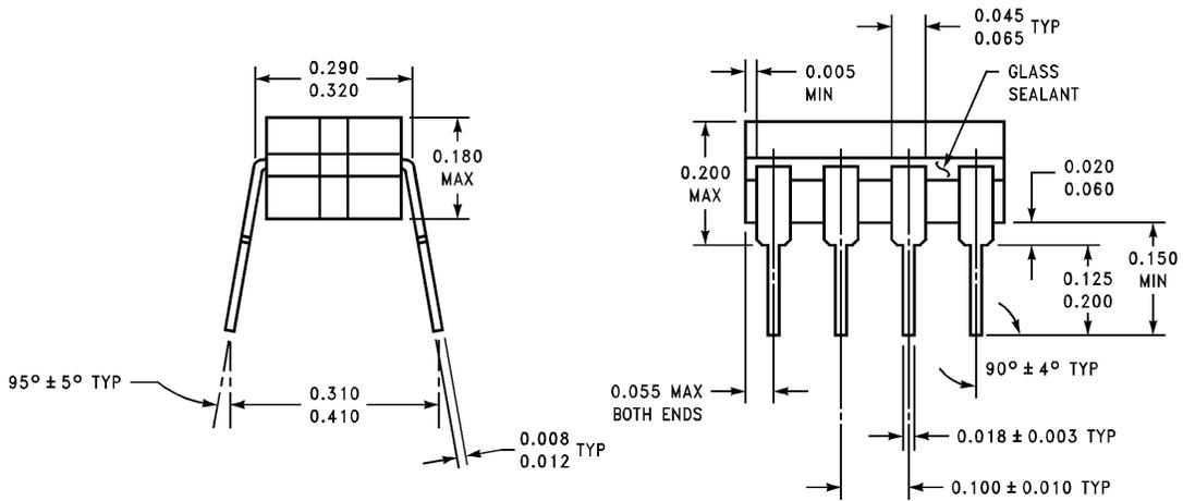
**8-Pin Ceramic Dual-In-Line Package**
