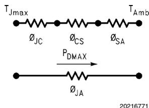
Once the maximum package power has been calculated using Equation 2, the maximum thermal resistance,  $\theta_{SA}$ , (heat sink to ambient) in  $^{\circ}\text{C}/\text{W}$  for a heat sink can be calculated. This calculation is made using Equation 3 which is derived by solving for  $\theta_{SA}$  from Equation 2.
