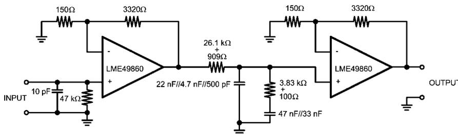
Note: 1% metal film resistors, 5% polypropylene capacitors
