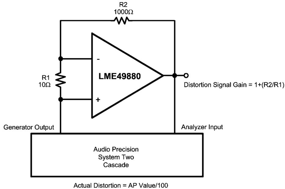
**FIGURE 7: THD+N and IMD Distortion Test Circuit**
