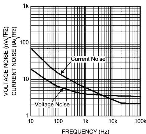
FIGURE 1: Current Noise and Voltage Spectral Density
