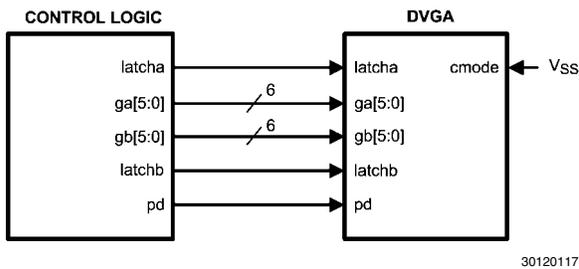
FIGURE 7. Parallel Mode Connection for Fastest Response
