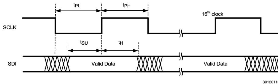
FIGURE 13. Write Timing
