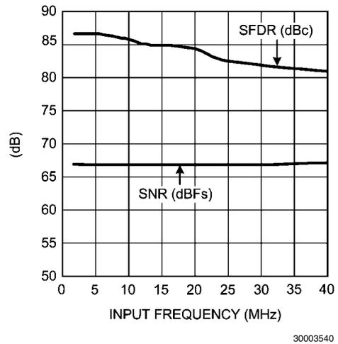
**FIGURE 8. LMH6552/ADC12DL080 SFDR and SNR Performance vs. Frequency**
