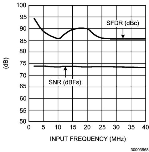
FIGURE 10. LMH6552/ADC14DS105 SFDR and SNR Performance vs. Frequency
