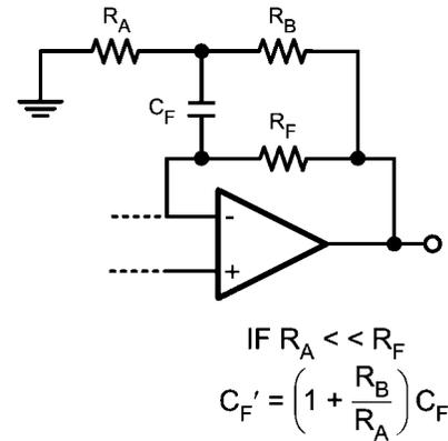
**FIGURE 7. Modified Transimpedance Amplifier**
