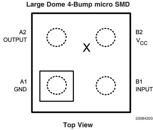
**Note:** - Pin numbers are referenced to package marking text orientation.
