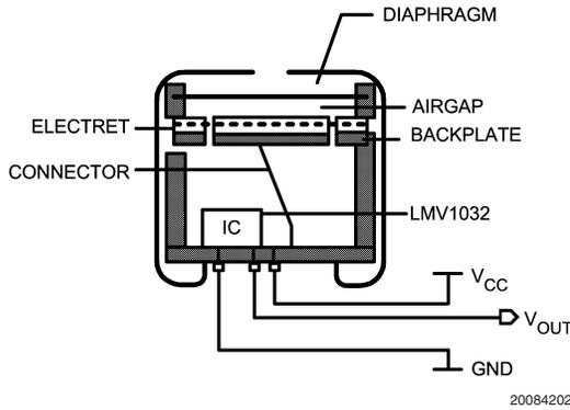
FIGURE 1. Built-in Gain
