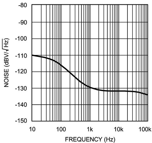
**Output Voltage Noise vs. Frequency (LMV1032-25)**
