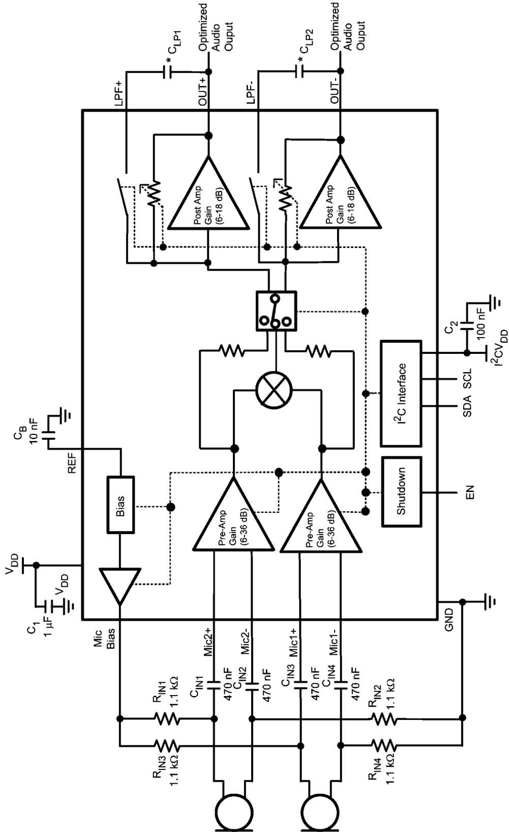
\* The value of the low-pass filter capacitor is application dependent, see the application section for additional information.
