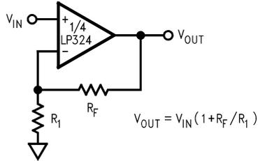
$$V_{OUT} = V_{IN} (1 + R_F / R_1)$$
