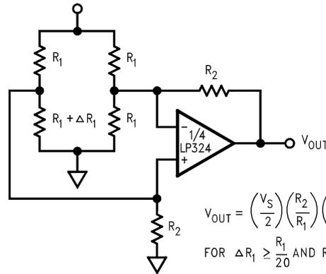
$$V_{OUT} = \left(\frac{V_S}{2}\right) \left(\frac{R_2}{R_1}\right) \left(\frac{\Delta R_1}{R_1}\right)$$
