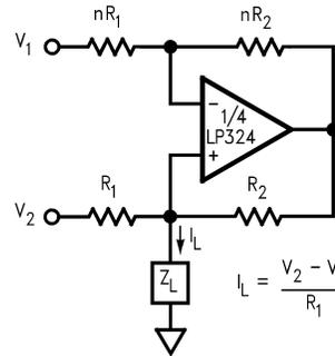
$$I_L = \frac{V_2 - V_1}{R_1}$$
