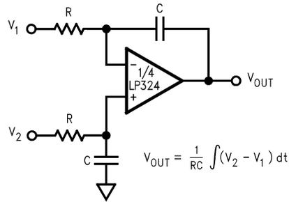
$$V_{OUT} = \frac{1}{RC} \int (V_2 - V_1) dt$$
