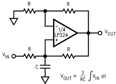
$$V_{OUT} = \frac{2}{RC} \int V_{IN} dt$$
