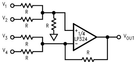
$$V_{OUT} = V_1 + V_2 - V_3 - V_4$$
