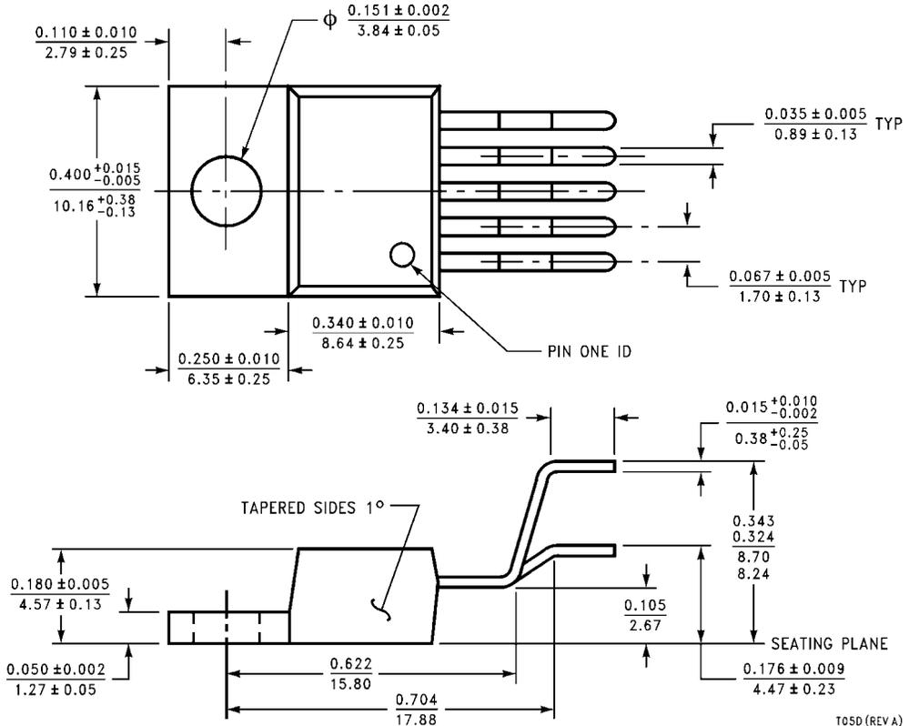
**TO220 5-lead, Molded, Stagger Bend Package (TO220-5)
