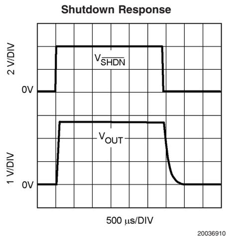
**Typical Performance Characteristics** Unless otherwise specified,  $V_{IN} = V_O + 0.5V$ ,  $C_{IN} = C_{OUT} = 2.2\mu F$ ,  $C_{CC} = 33nF$ ,  $T_J = 25^\circ C$ ,  $V_{SHDN} = V_{IN}$ . (Continued)
