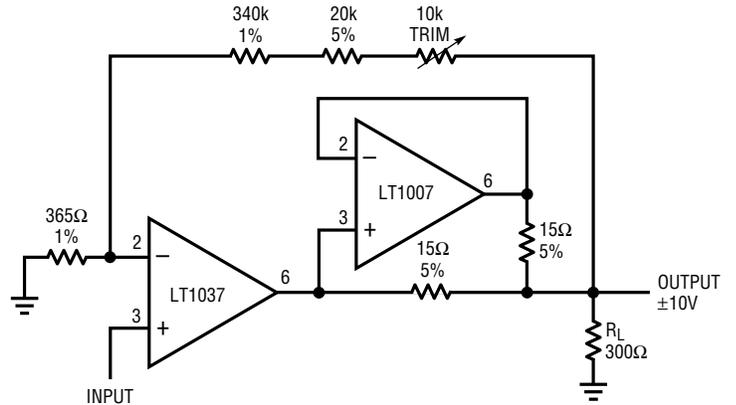
THE ADDITION OF THE LT1007 DOUBLES THE AMPLIFIER'S OUTPUT DRIVE TO ±33mA. GAIN ACCURACY IS 0.02%, SLIGHTLY DEGRADED COMPARED TO ABOVE BECAUSE OF SELF-HEATING OF THE LT1037 UNDER LOAD.
