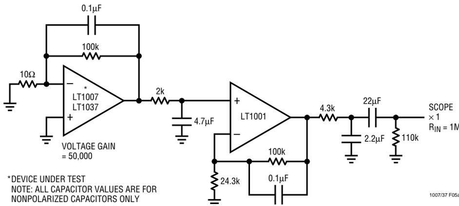
Figure 5a. 0.1Hz to 10Hz Noise Test Circuit
