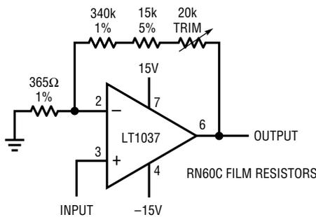
THE HIGH GAIN AND WIDE BANDWIDTH OF THE LT1037 (AND LT1007) IS USEFUL IN LOW FREQUENCY, HIGH CLOSED-LOOP GAIN AMPLIFIER APPLICATIONS. A TYPICAL PRECISION OP AMP MAY HAVE AN OPEN-LOOP GAIN OF ONE MILLION WITH 500kHz BANDWIDTH. AS THE GAIN ERROR PLOT SHOWS, THIS DEVICE IS CAPABLE OF 0.1% AMPLIFYING ACCURACY UP TO 0.3Hz ONLY. EVEN INSTRUMENTATION RANGE SIGNALS CAN VARY AT A FASTER RATE. THE LT1037'S "GAIN PRECISION-BANDWIDTH PRODUCT" IS 200 TIMES HIGHER AS SHOWN.
