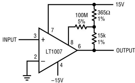
POSITIVE FEEDBACK TO ONE OF THE NULLING TERMINALS CREATES APPROXIMATELY 5μV OF HYSTERESIS. OUTPUT CAN SINK 16mA.
