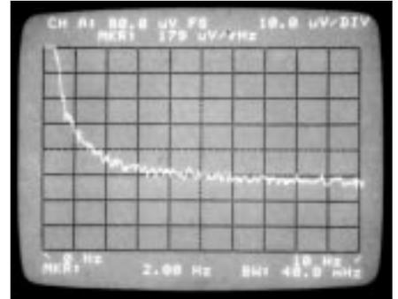
MARKER AT 2Hz (= 1/f CORNER) =  $\frac{179\mu\text{V}/\sqrt{\text{Hz}}}{50,000} = 3.59 \frac{\text{nV}}{\sqrt{\text{Hz}}}$
