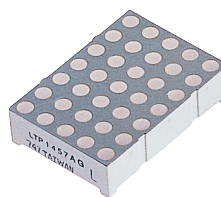
31.79mm (3 \phi ) Dual-In-Line 1.25"H x .9"W x .31"D
