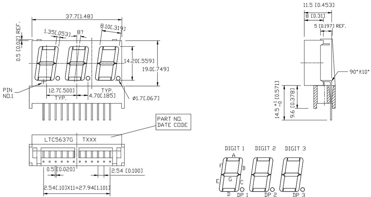
NOTES: All dimensions are in millimeters. Tolerances are ± 0.25 mm (0.01") unless otherwise noted.
