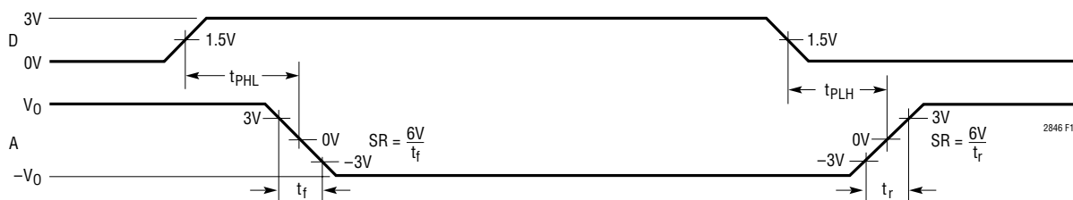
Figure 15. V.28 Driver Propagation Delays
