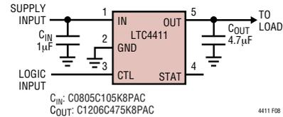
Figure 8. Logic Controlled High Side Power Switch
