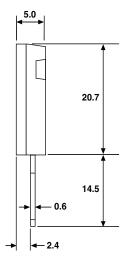
$<sup>\</sup>bullet$  Tolerance unless otherwise specified:  $\pm$  0.3 mm
