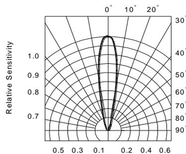
FIG.5 SENSITIVITY DIAGRAM
