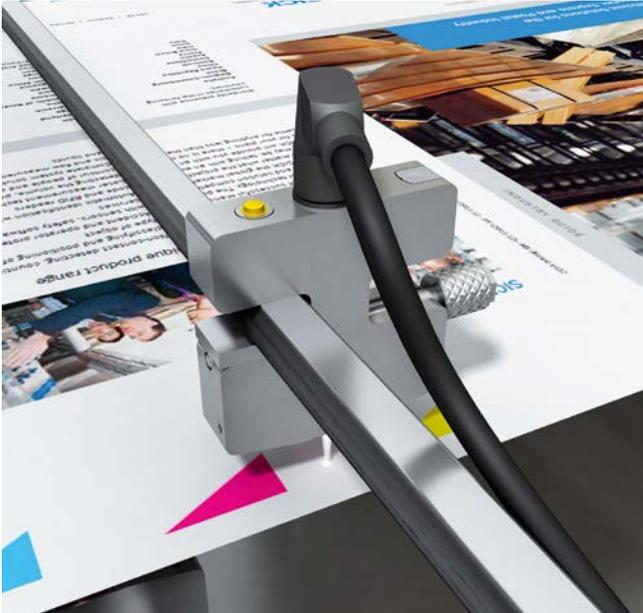
The RS10 register sensor is perfect for detecting minor contrasts and lots of different colors. With an integrated register control system and configurable individual switching threshold, a sensor can detect up to 18 marks.
