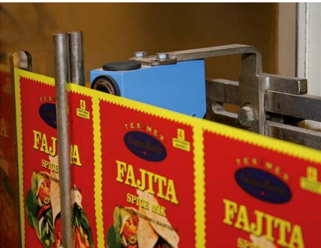
The size of the color sensor's light spot depends on the sensing distance.
