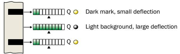
Fine adjustment possible using the "+" / "-" buttons.
