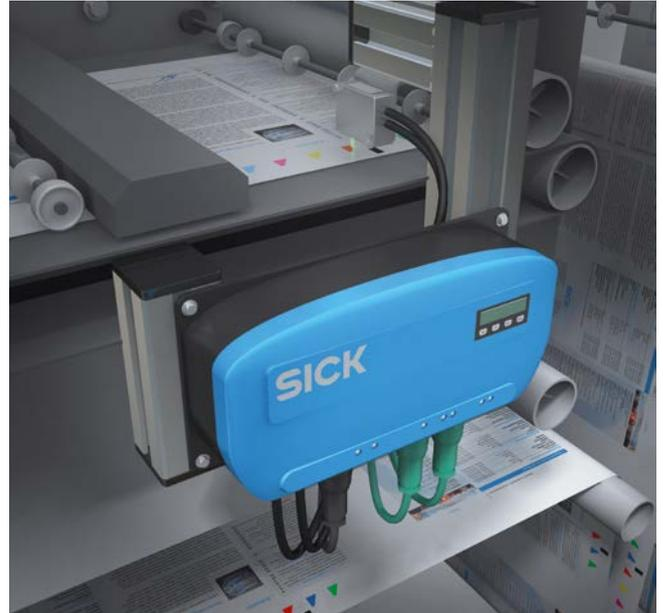
The RS25 register sensor is impressively simple and quick to use and features automatic teach-in mechanisms. This reduces machine setup and conversion times. It consists of a sensor head, fibers, and evaluation unit. Using an RGB light ensures excellent reading quality.
