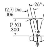
**Standard Combinations:** S4 Bat Lever with bracketed terminals (codes 13, 30, 40) with silver or gold contacts.
