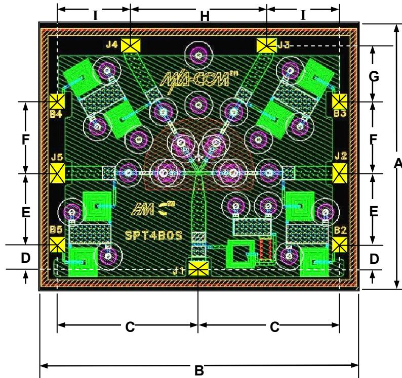
5. Topside and backside metallization is gold, 2.5  $\mu$ m thick typical.
