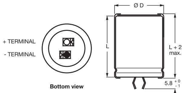
The minus terminal can be marked with a black dot or with an imprinted “-” sign.
