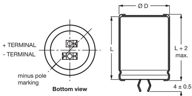
The negative terminal has **TWO** pins which are **BOTH** electrically connected.
