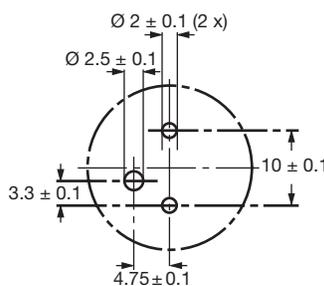
The 10 mm spacing of the 2 pin snap-in is used as the base layout and a third hole is added.
