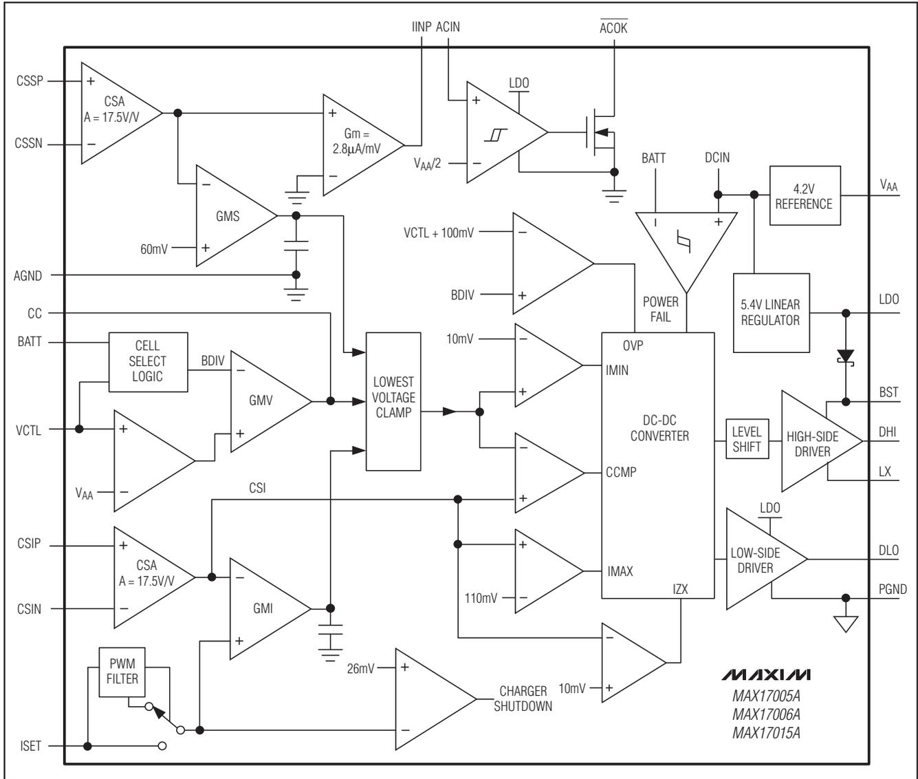
Figure 2. Functional Diagram
