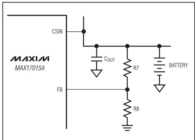
Figure 3. The MAX17015A Charge-Voltage Regulation Feedback Network
