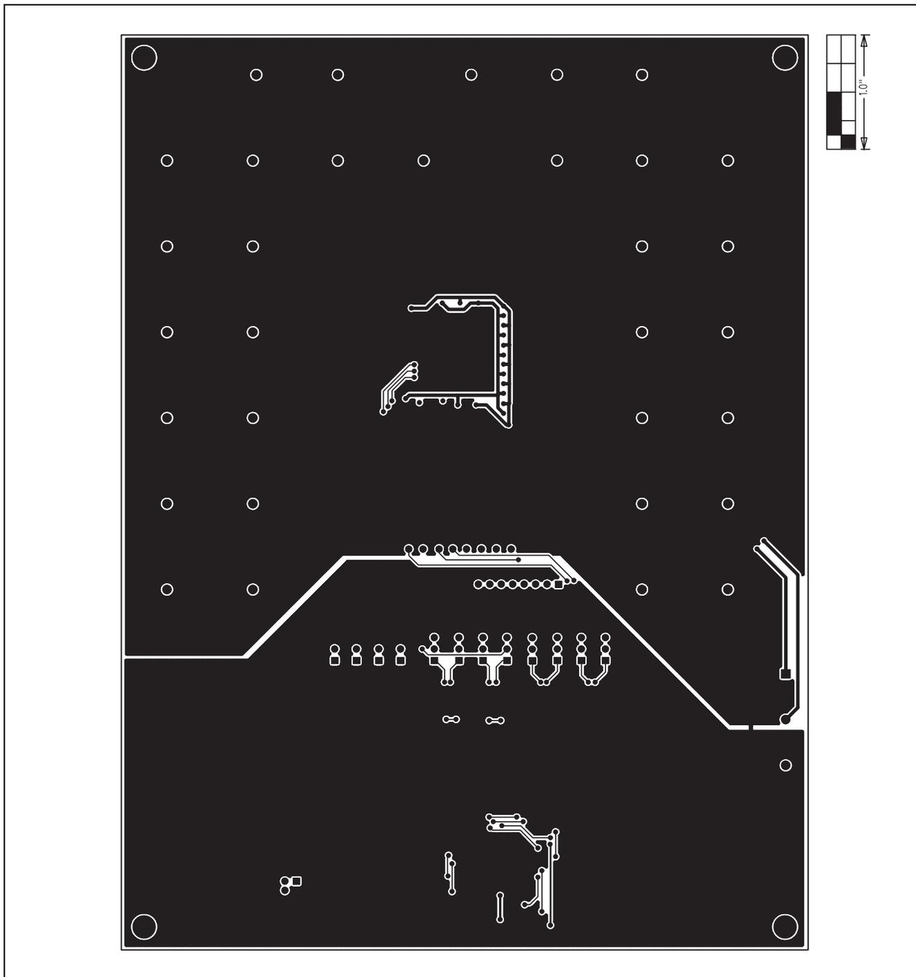
Figure 6. MAX9675 EV Kit PCB Layout—Solder Side
