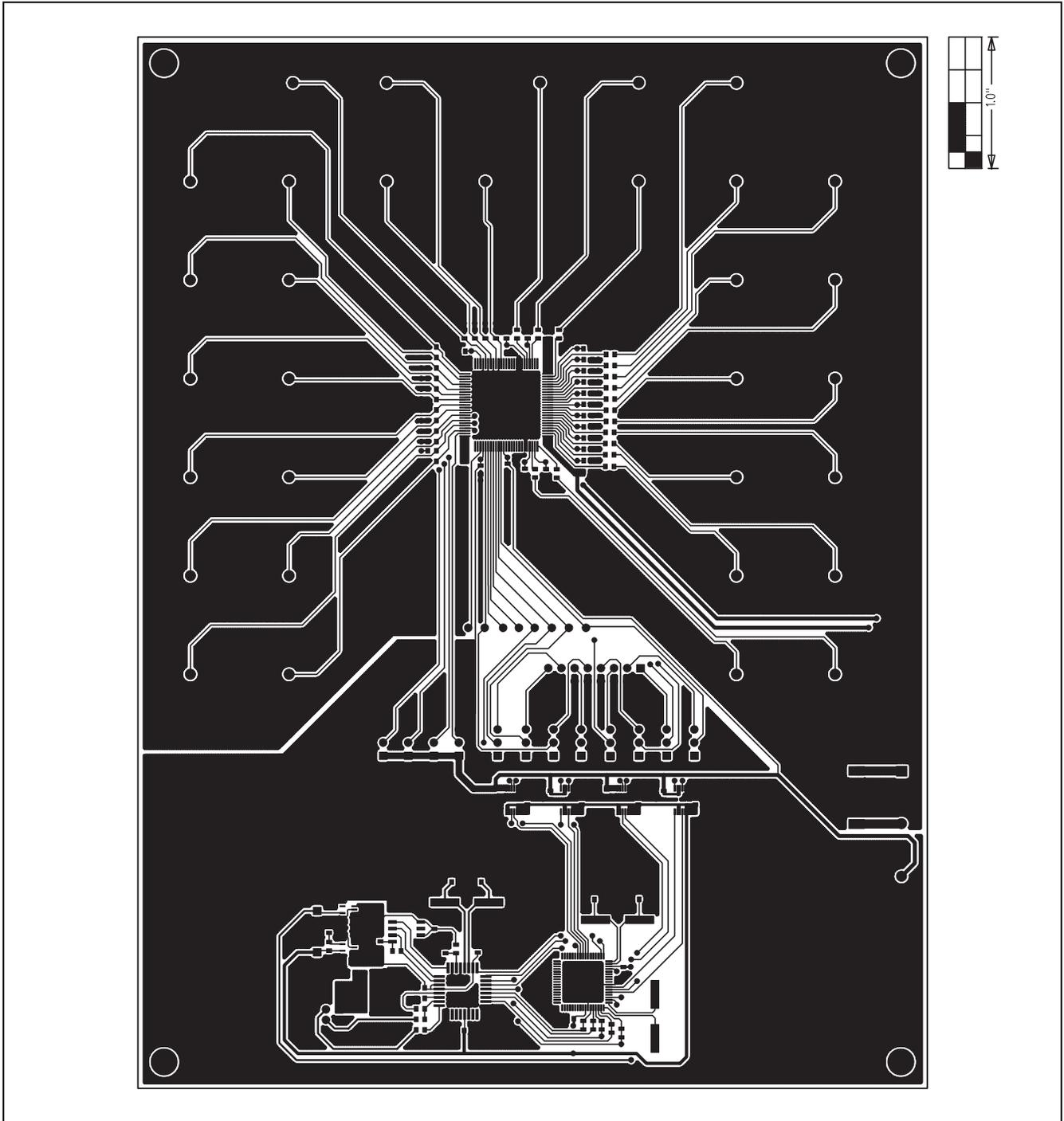
Figure 5. MAX9675 EV Kit PCB Layout—Component Side
