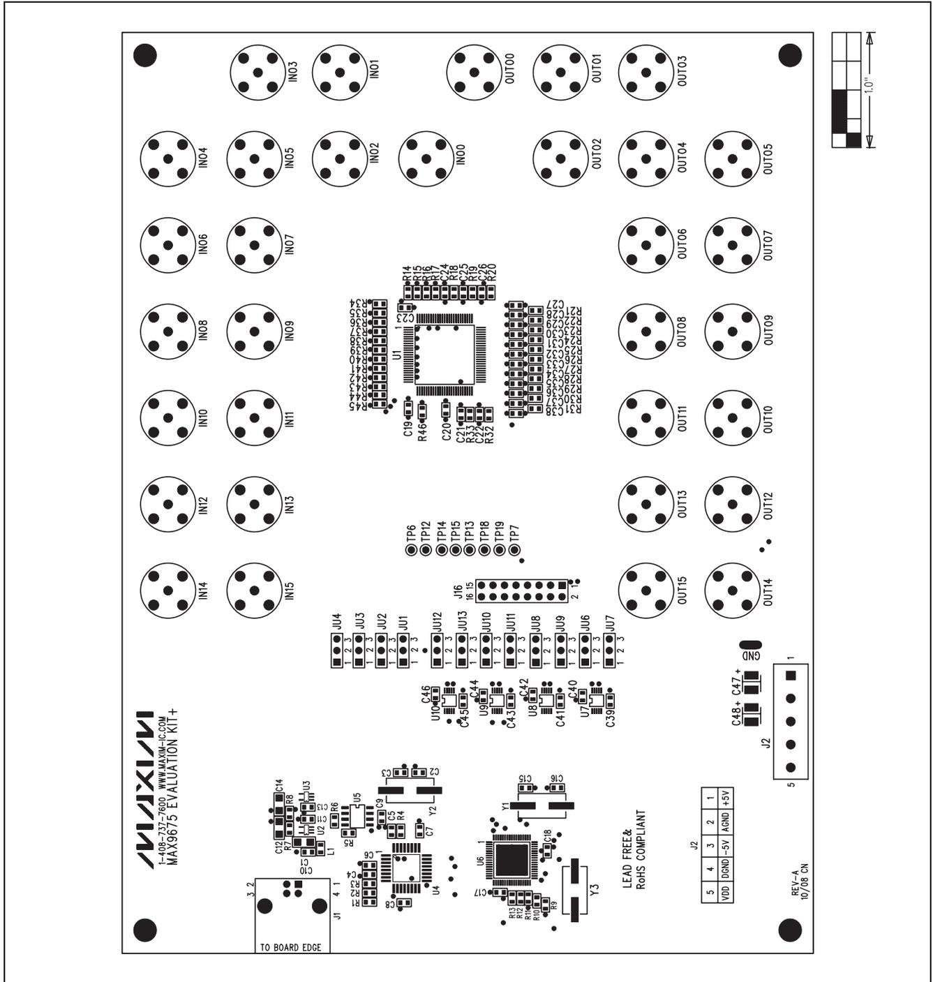
Figure 4. MAX9675 EV Kit Component Placement Guide—Component Side
