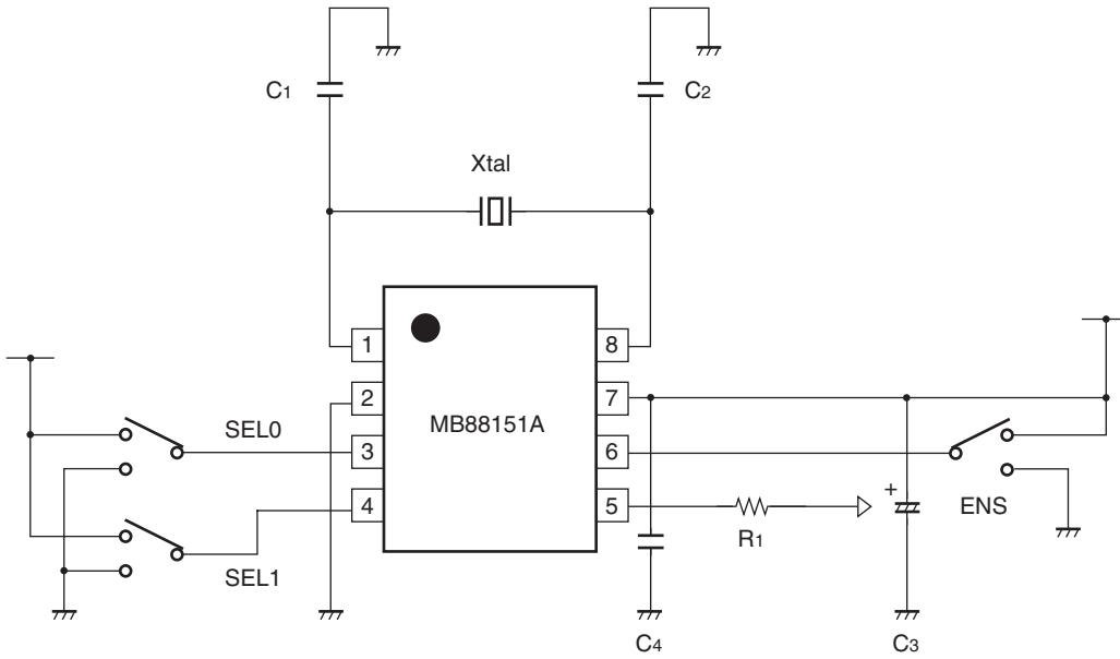
C<sub>1</sub>, C<sub>2</sub> : Oscillation stabilization capacitance (refer to "OSCILLATION CIRCUIT".)
