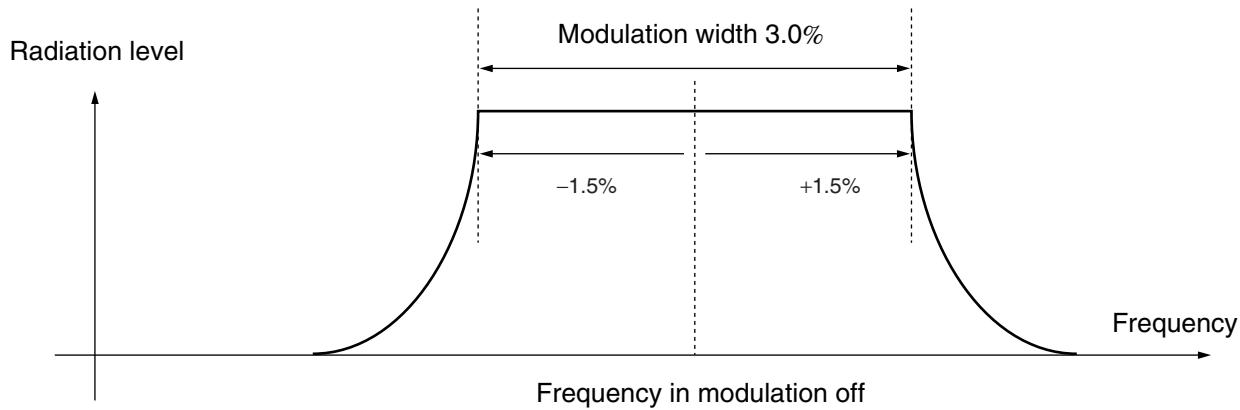
Center spread example of  $\pm 1.5\%$  modulation rate
