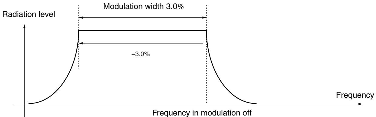
Down spread example of  $-3.0\%$  modulation rate
