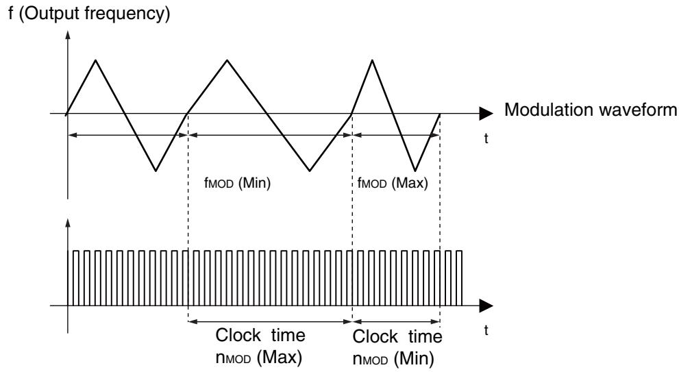
MB88151A contains the modulation period to realize the efficient EMI reduction.
