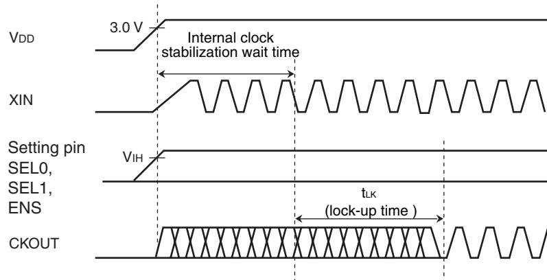
If the setting pin is fixed at the "H" or "L" level, the maximum time after the power is turned on until the set clock signal is output from CKOUT pin is (the stabilization wait time of input clock to XIN pin) + (the lock-up time "t<sub>LK</sub>"). For the input clock stabilization time, check the characteristics of the resonator or oscillator used.
