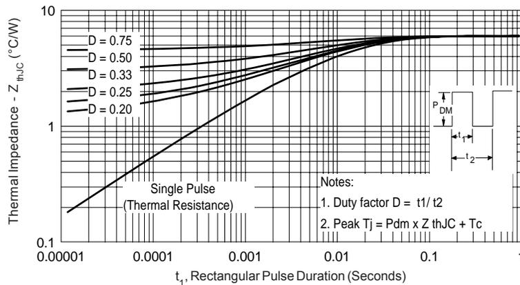
Fig. 4 - Max. Thermal Impedance  $Z_{thJC}$  Characteristics (Per Leg)
