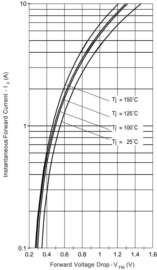
Fig. 1 - Max. Forward Voltage Drop Characteristics (Per Leg)
