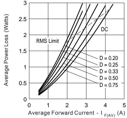
Fig. 6 - Forward Power Loss Characteristics (Per Leg)
