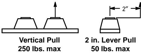
Note: While the POWERTAP is capable of sustaining these vertical and levered tensions, the intimate contact between POWERTAP and heat sink may be lost. This could lead to thermal runaway. The use of very flexible leads is recommended for the anode connections. Use of thermal grease is highly recommended.
