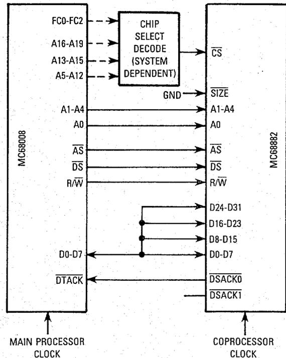
Figure 15. 8-Bit Data Bus Peripheral Processor Connection
