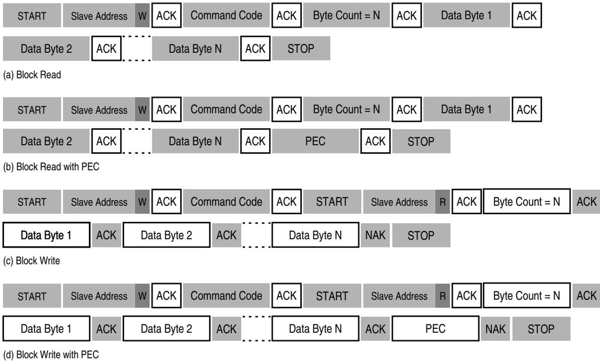
Figure 14-19. Block Read/Write
