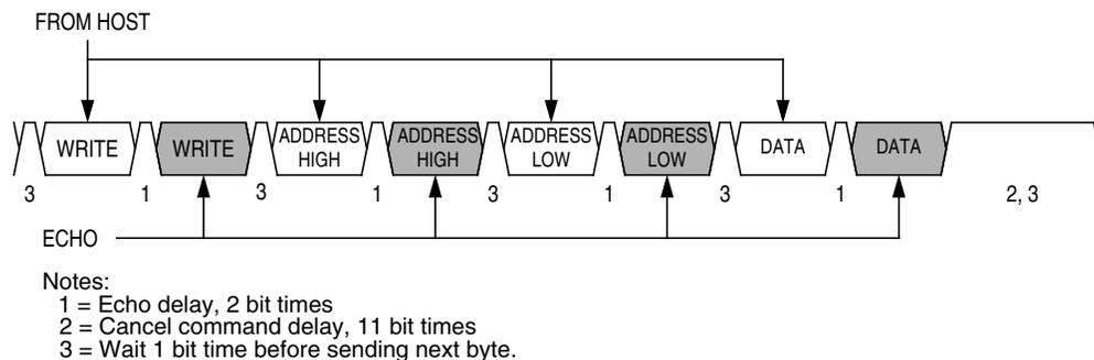
**Figure 8-6. Write Transaction**
