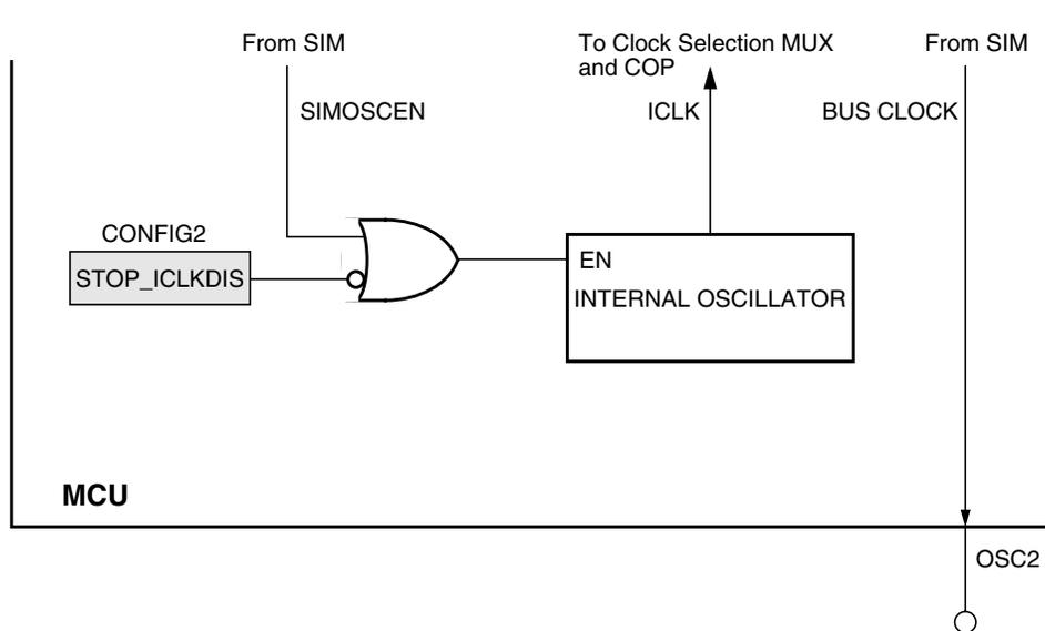
Figure 5-4. Internal Oscillator
