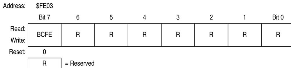
**Figure 21-7. SIM Break Flag Control Register (SBFCR)**
