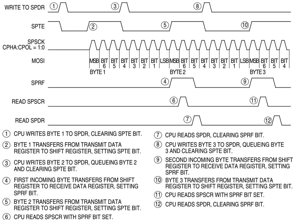
**Figure 13-8. SPRF/SPTe CPU Interrupt Timing**
