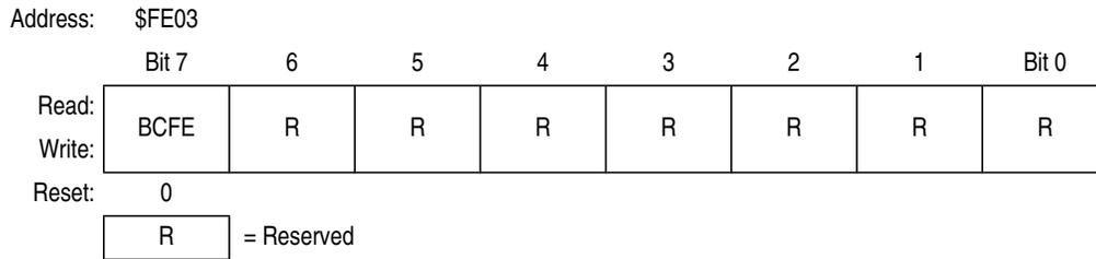
**Figure 7-22. SIM Break Flag Control Register (SBFCR)**
