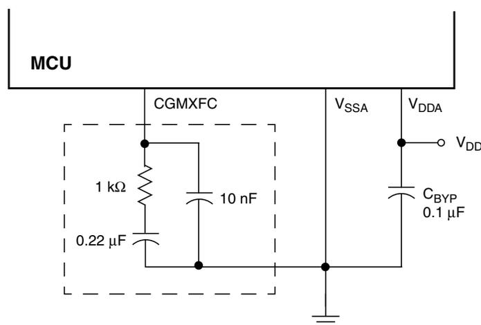
Note: Filter network in box can be replaced with a 0.47  $\mu$ F capacitor, but will degrade stability.
