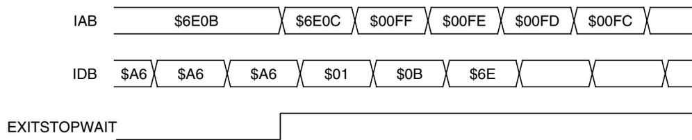
NOTE: EXITSTOPWAIT =  $\overline{\text{RST}}$  pin OR CPU interrupt OR break interrupt
