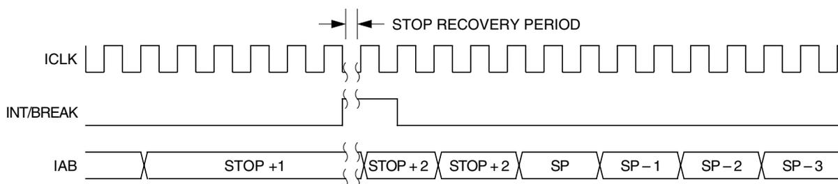
**Figure 7-19. Stop Mode Recovery from Interrupt or Break**
