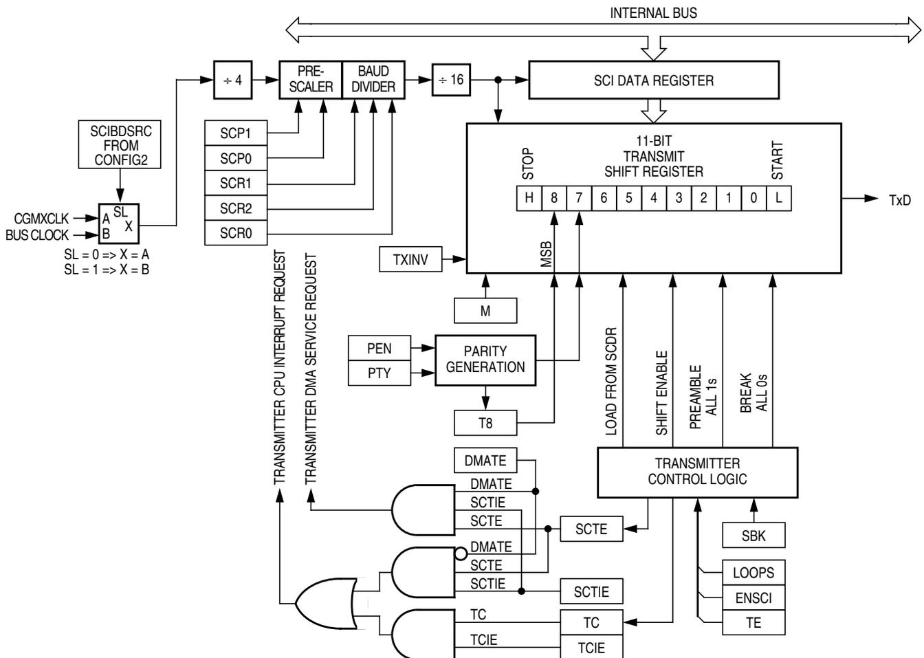
Figure 11-4. SCI Transmitter
