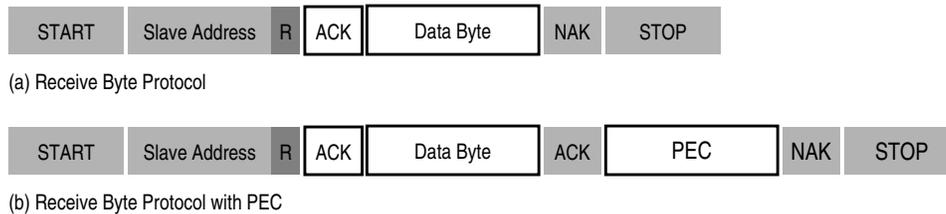
**Figure 14-15. Receive Byte**
