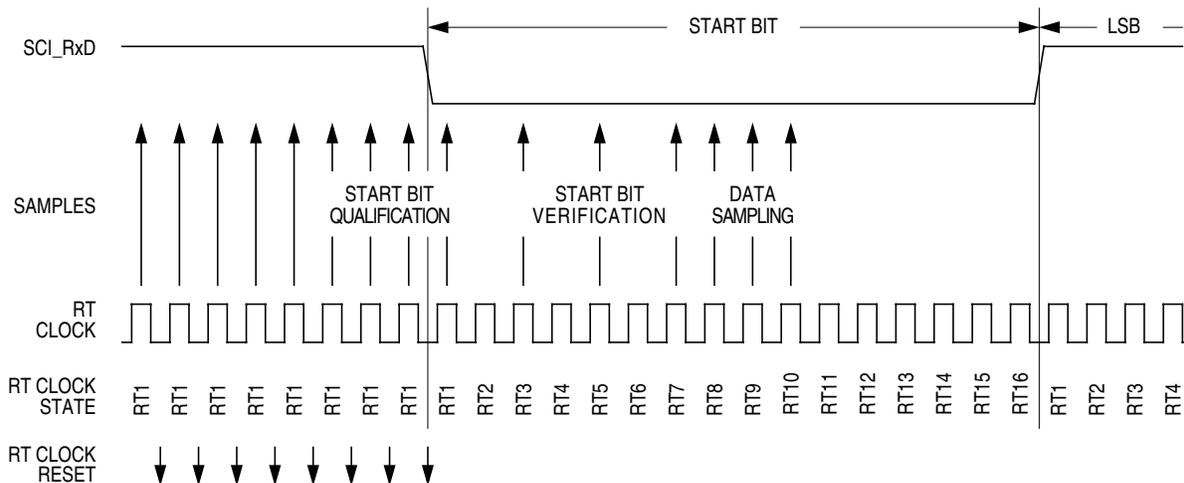
Figure 12-9. Receiver Data Sampling
