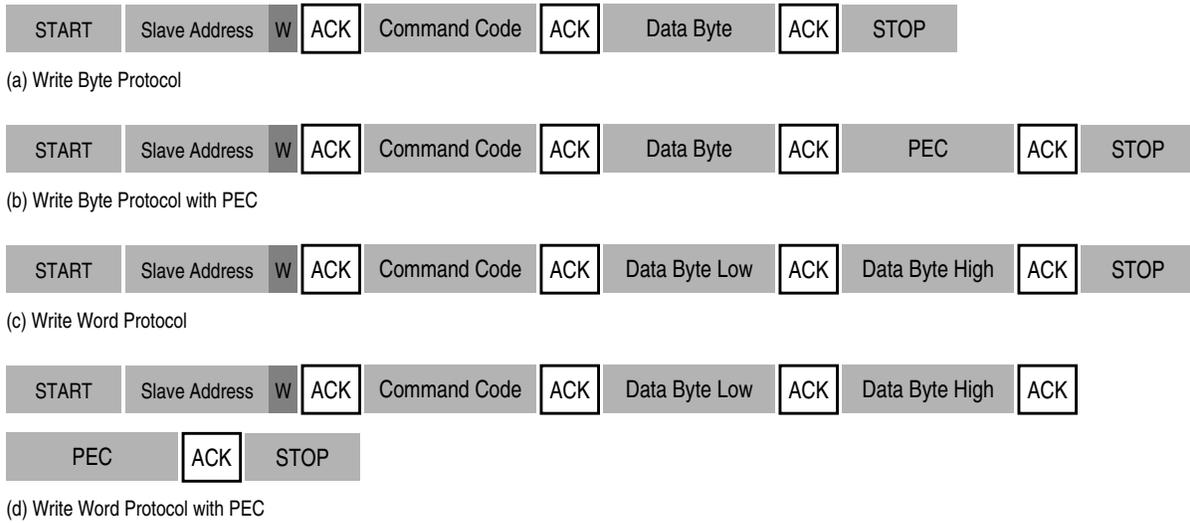
Figure 14-16. Write Byte/Word
