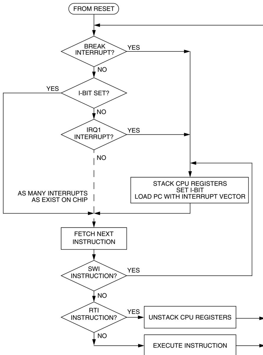
**Figure 7-10. Interrupt Processing**
