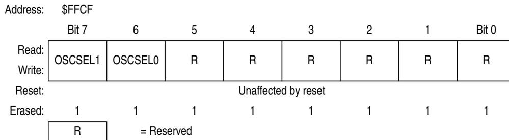
**Figure 3-4. Mask Option Register (MOR)****OSCSEL1, OSCSEL0 — Oscillator Selection Bits**
