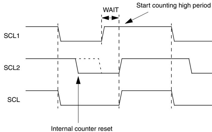
**Figure 14-3. Clock Synchronization**
