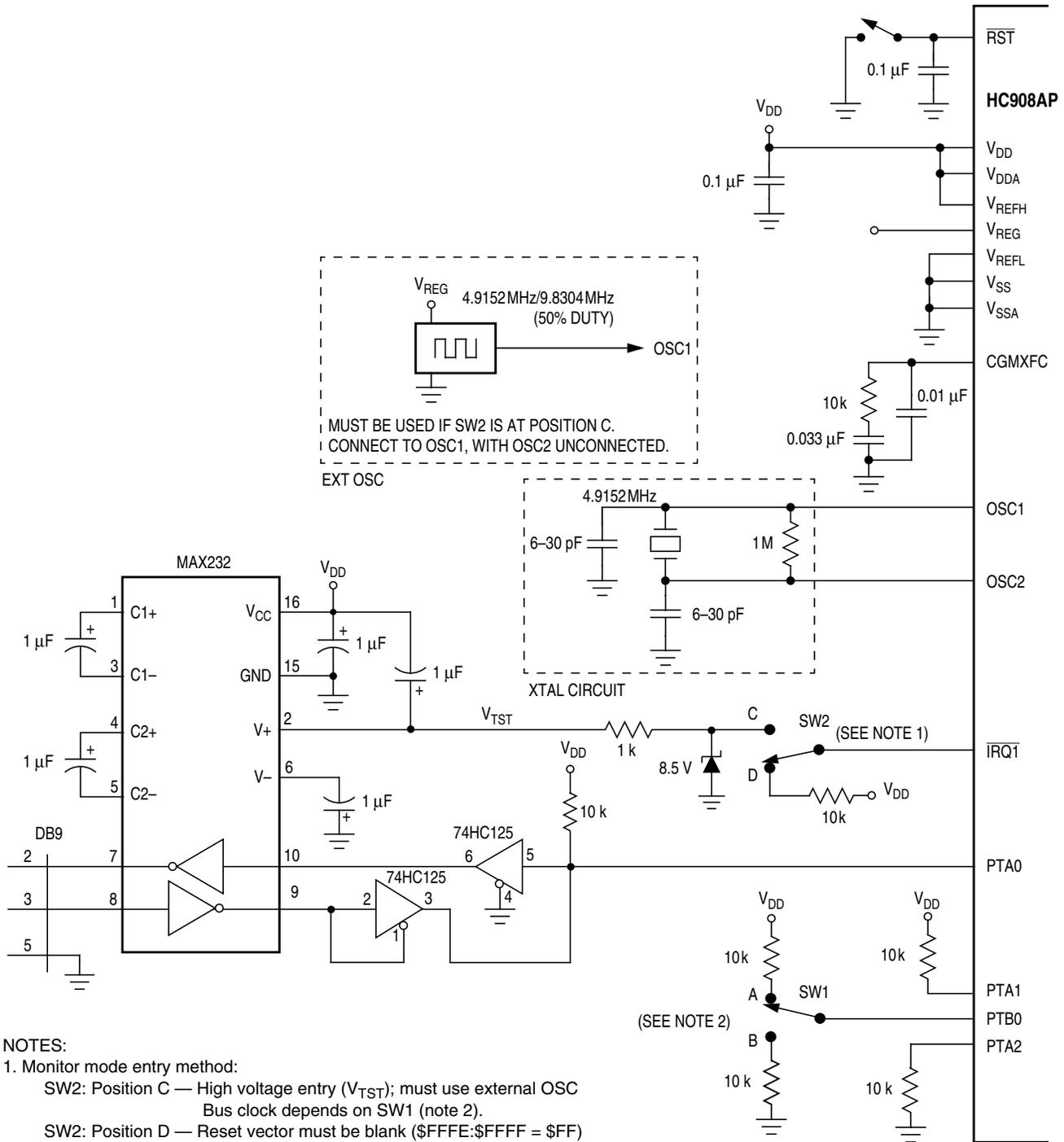
Figure 8-1. Monitor Mode Circuit
