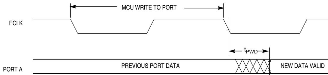
**Figure 20-7. Port Write Timing Diagram**
