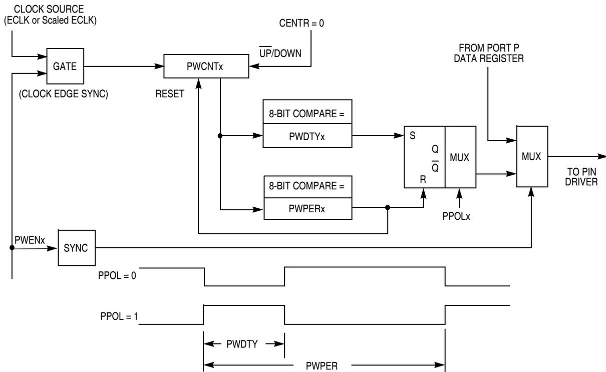
**Figure 13-1. Block Diagram of PWM Left-Aligned Output Channel**
