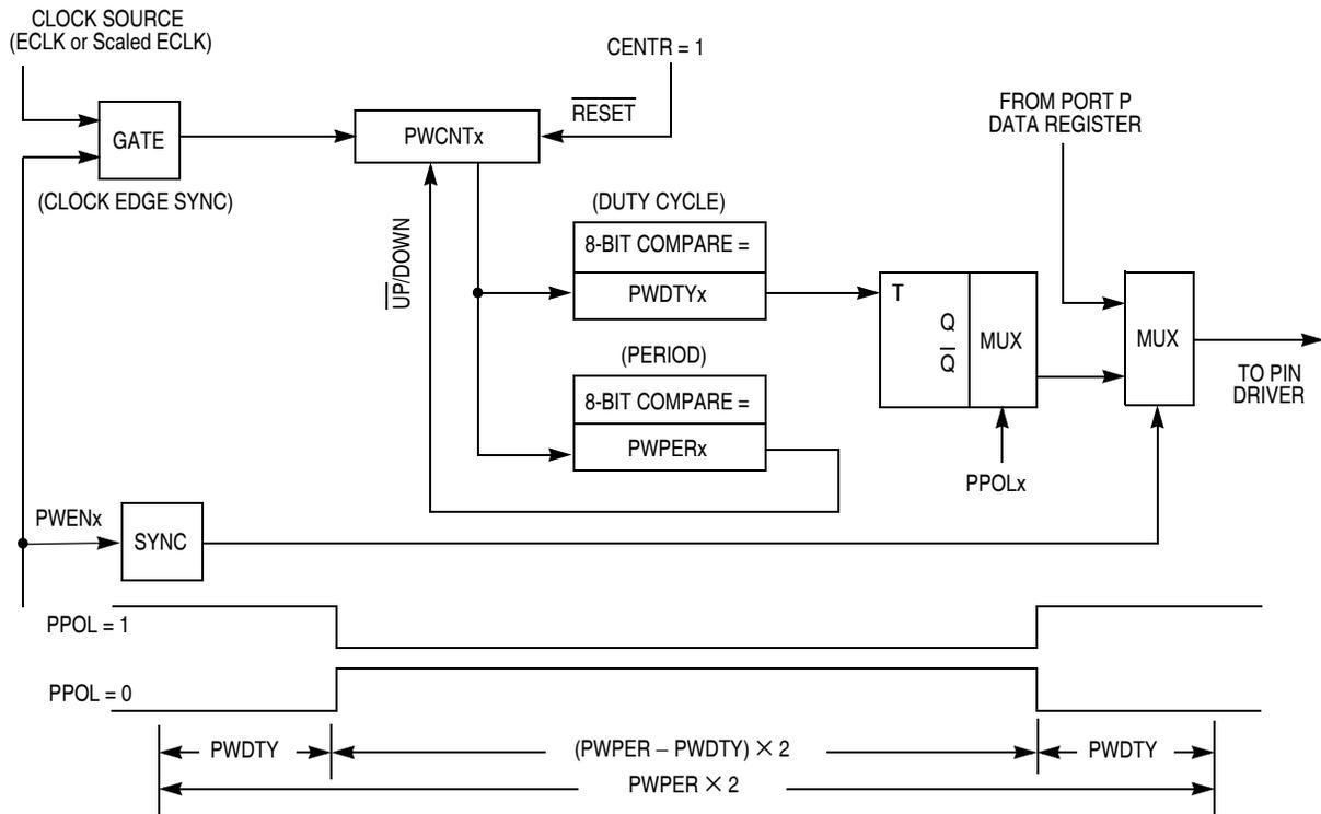
**Figure 13-2. Block Diagram of PWM Center-Aligned Output Channel**
