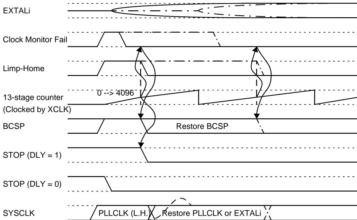
**Figure 11-5. STOP Exit and Fast STOP Recovery**
