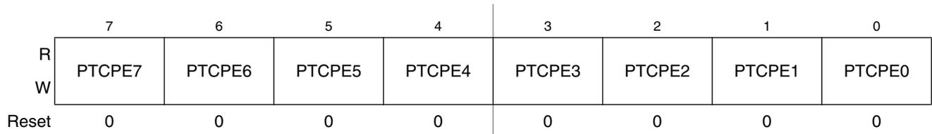
Figure 6-17. Pullup Enable for Port C (PTCPE)
