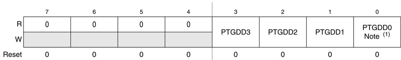
Figure 6-31. Data Direction for Port G (PTGDD)
