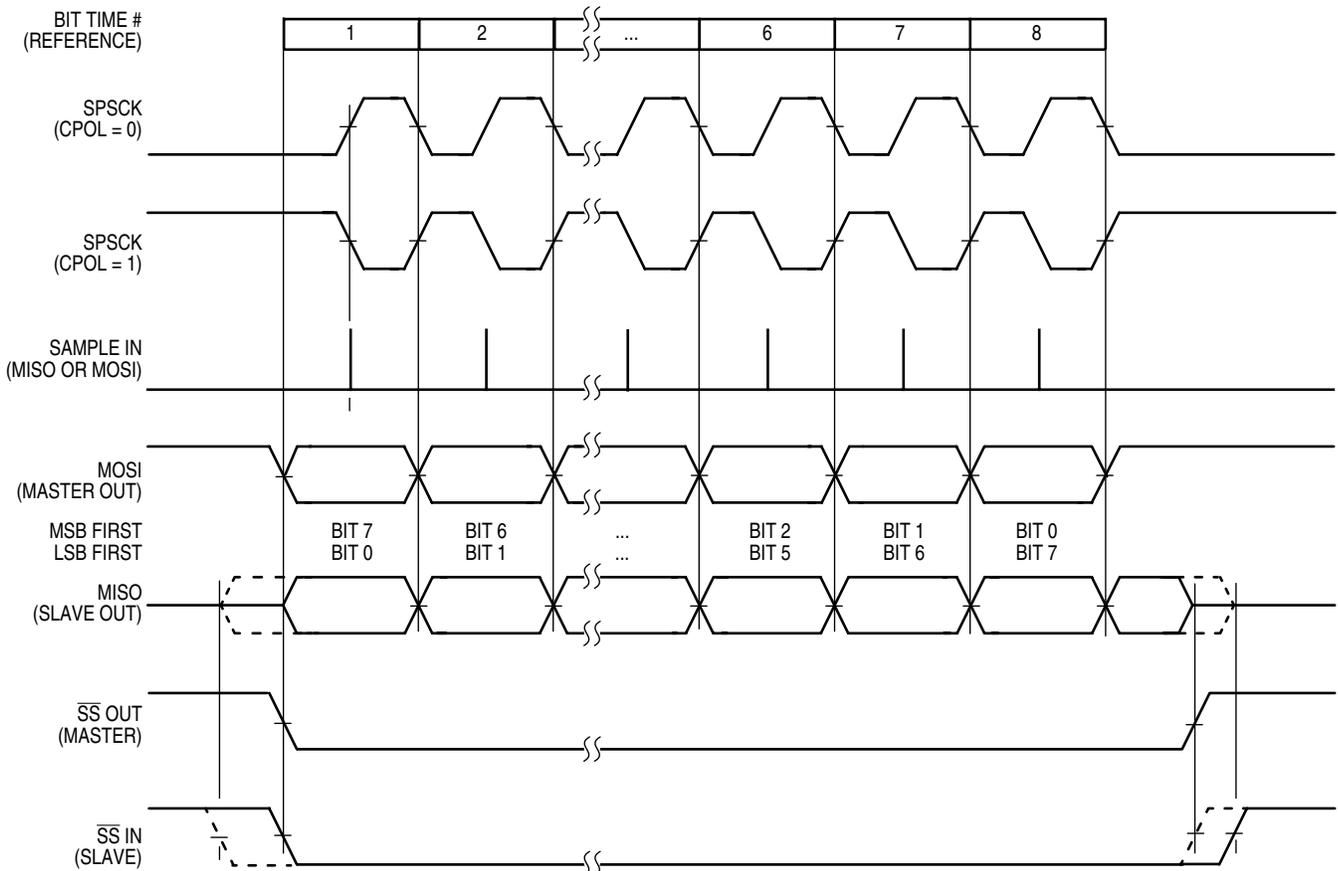
Figure 12-12. SPI Clock Formats (CPHA = 0)
