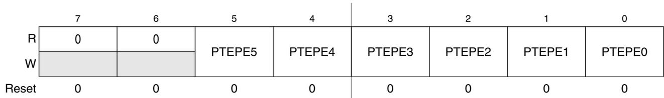
**Figure 6-25. Pullup Enable for Port E (PTEPE)**
