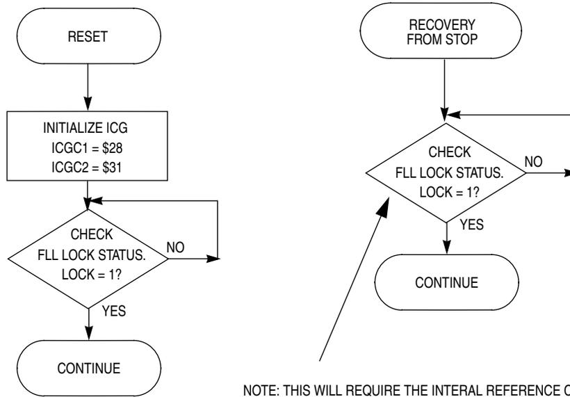
Figure 9-16. ICG Initialization and Stop Recovery for Example #3
