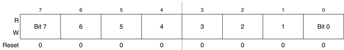
**Figure 10-7. Timer x Counter Modulo Register Low (TPMxMODL)**
