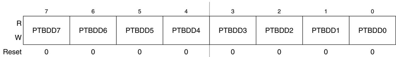
Figure 6-15. Data Direction for Port B (PTBDD)
