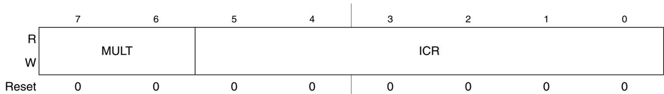
Figure 13-4. IIC Frequency Divider Register (IICF)
