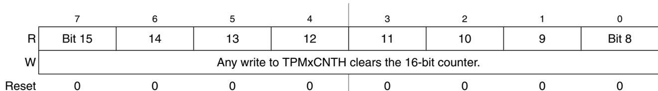
Figure 10-4. Timer x Counter Register High (TPMxCNTH)
