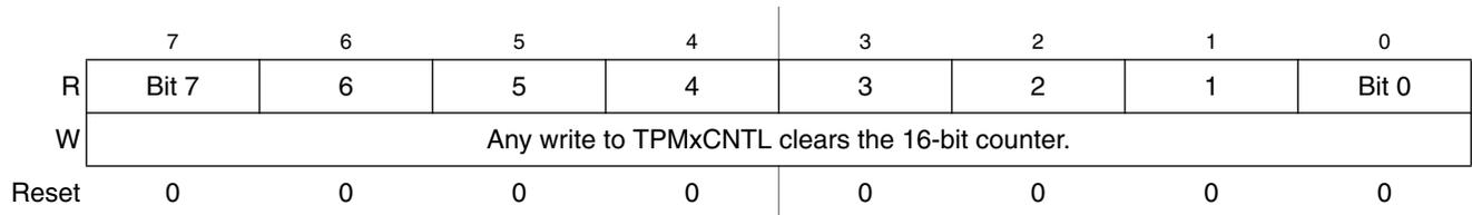
**Figure 10-5. Timer x Counter Register Low (TPMxCNTL)**
