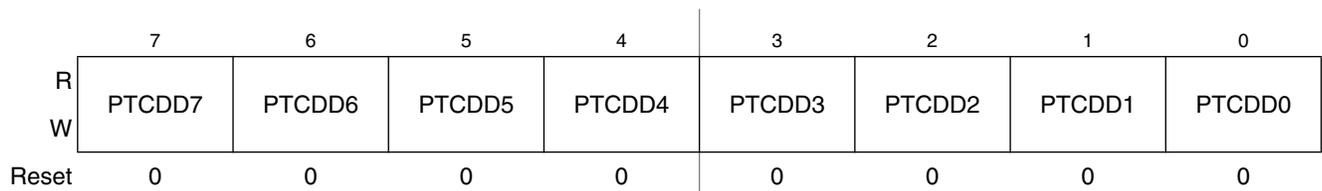
Figure 6-19. Data Direction for Port C (PTCDD)
