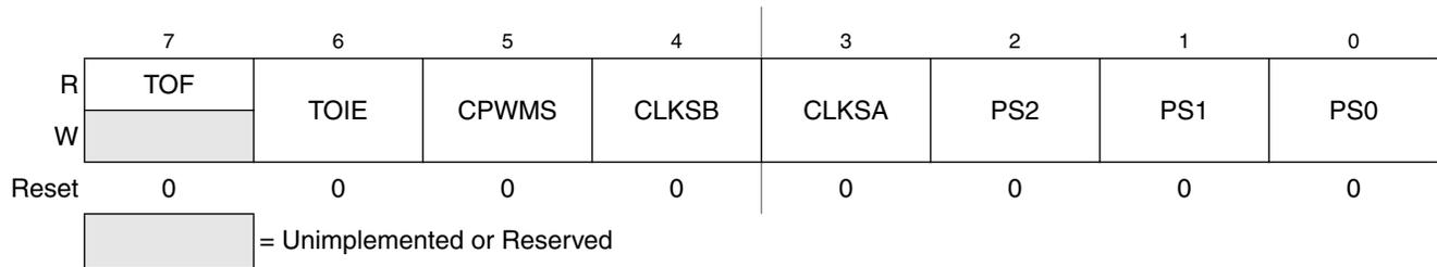
**Figure 10-3. Timer x Status and Control Register (TPMxSC)**
