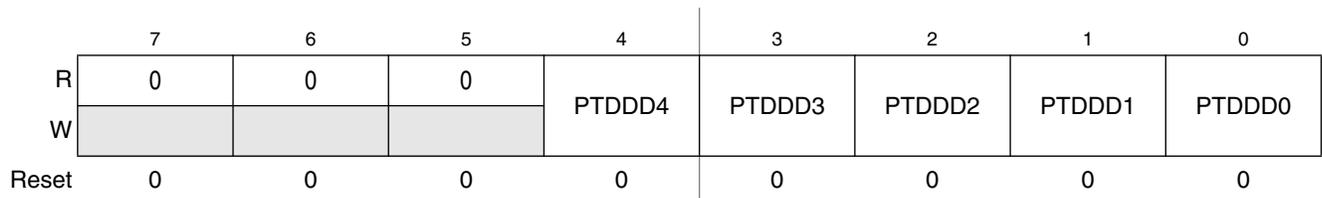
Figure 6-23. Data Direction for Port D (PTDDD)
