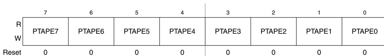
Figure 6-9. Pullup Enable for Port A (PTAPE)
