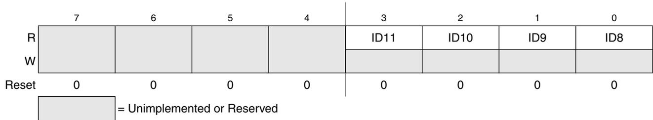
**Figure 5-6. System Device Identification Register High (SDIDH)**
