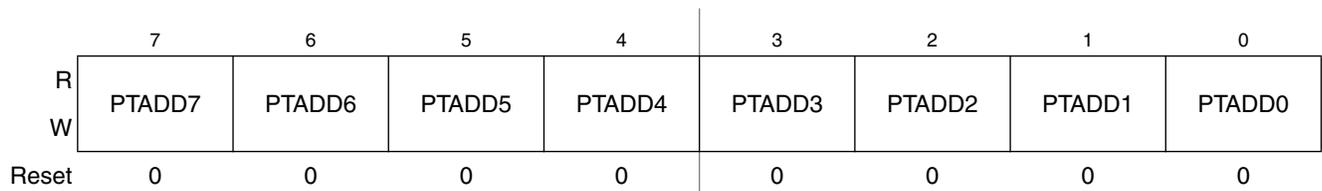
Figure 6-11. Data Direction for Port A (PTADD)
