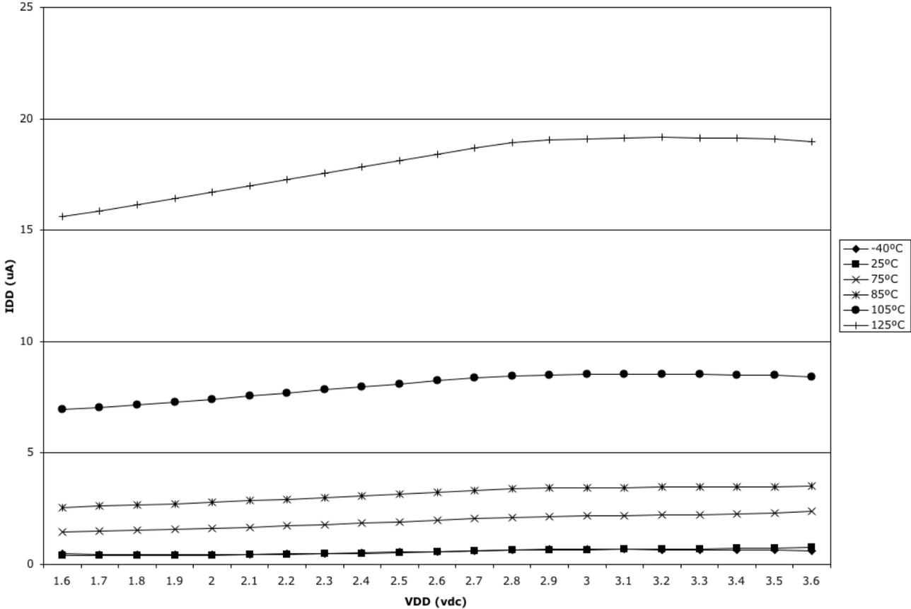
Figure A-9. Typical Stop3 I<sub>DD</sub>
