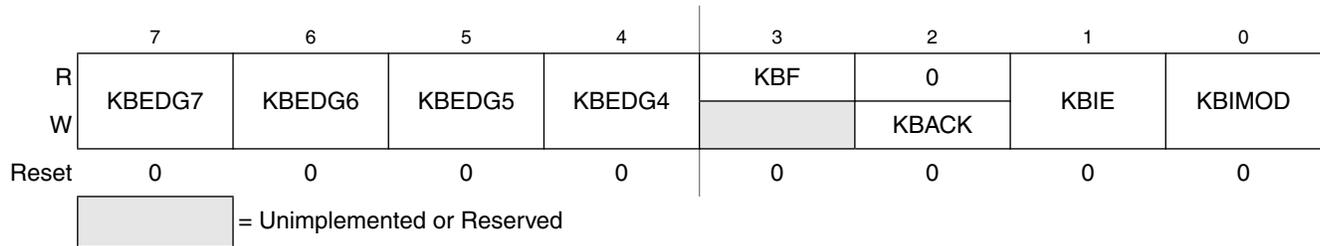
Figure 7-4. KBI Status and Control Register (KBISC)
