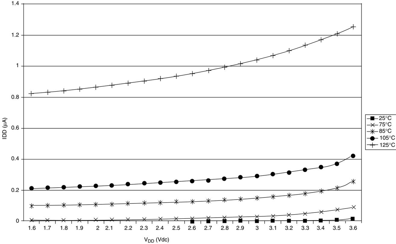
Figure A-7. Typical Stop1 I<sub>DD</sub>
