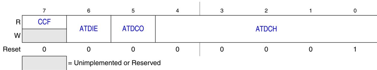
**Figure 14-6. ATD Status and Control Register (ATDSC)**
