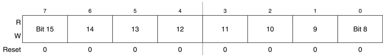
**Figure 10-6. Timer x Counter Modulo Register High (TPMxMODH)**
