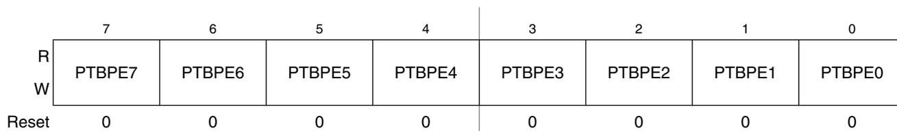
Figure 6-13. Pullup Enable for Port B (PTBPE)
