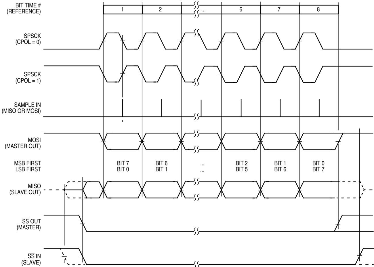
Figure 12-11. SPI Clock Formats (CPHA = 1)
