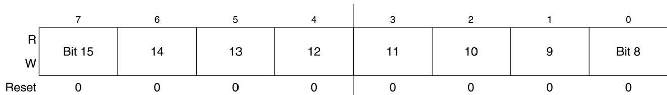
**Figure 10-9. Timer x Channel Value Register High (TPMxCnVH)**
