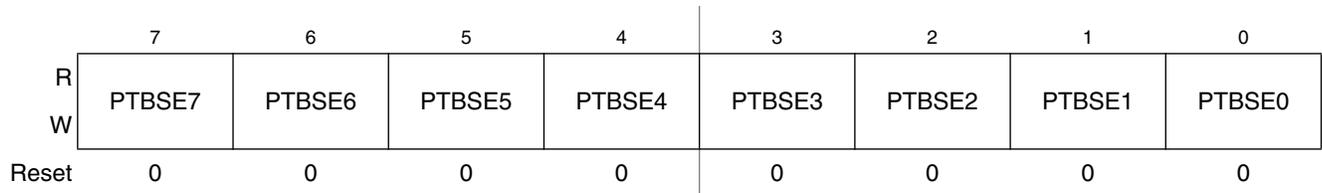
Figure 6-14. Data Direction for Port A (PTBSE)
