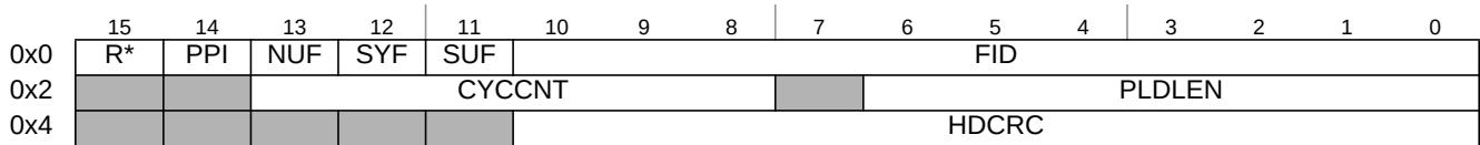
Figure 13-105. Frame Header Structure
