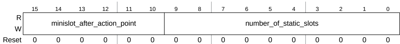
Figure 13-67. Protocol Configuration Register 2 (PCR2)
