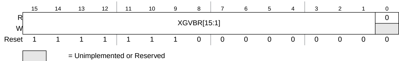
Figure 14-9. XGATE Vector Base Address Register (XGVBR)
