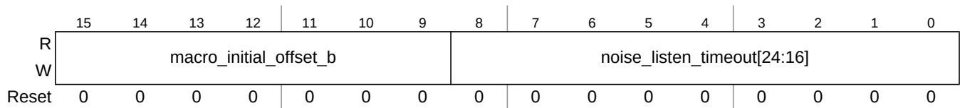
Figure 13-81. Protocol Configuration Register 16 (PCR16)
