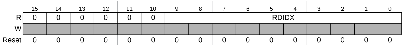
Figure 13-56. Receive FIFO B Read Index Register (RFBRIR)
