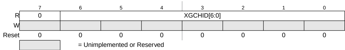
Figure 14-4. XGATE Channel ID Register (XGCHID)
