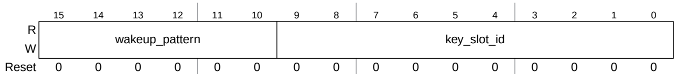
Figure 13-83. Protocol Configuration Register 18 (PCR18)
