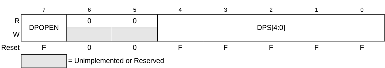
Figure 18-15. D-Flash Protection Register (DFPROT)
