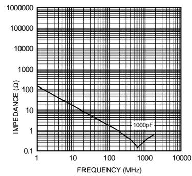
Fig.4 Impedance-frequency characteristics
