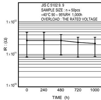
Fig.30 Insulation resistance
