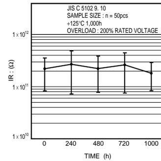
Fig.21 Insulation resistance
