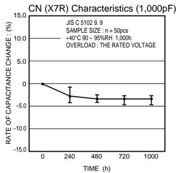
Fig.28 Rate of capacitance change
