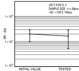
Fig.12 Insulation resistance
