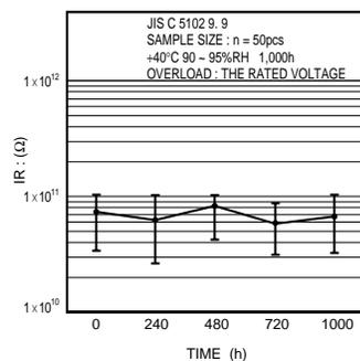
Fig.33 Insulation resistance
