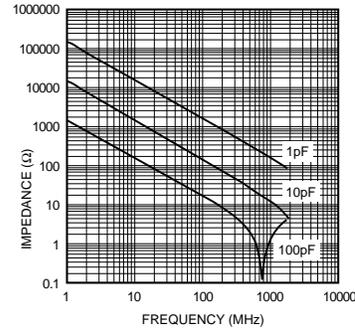
Fig.2 Impedance-frequency characteristics
