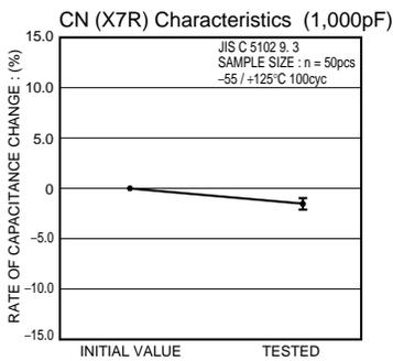
Fig.10 Rate of capacitance change
