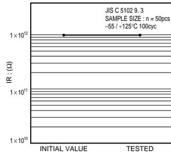
Fig.9 Insulation resistance
