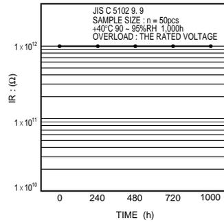
Fig.27 Insulation resistance
