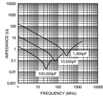
Fig.6 Impedance-frequency characteristics
