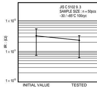
Fig.15 Insulation resistance
