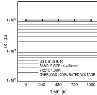
Fig.18 Insulation resistance
