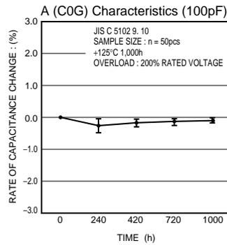
Fig.16 Rate of capacitance change
