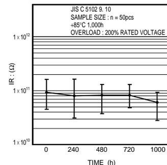
Fig.24 Insulation resistance
