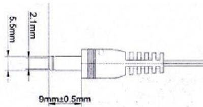
Figure 8. Plug size for DC5V power supply
