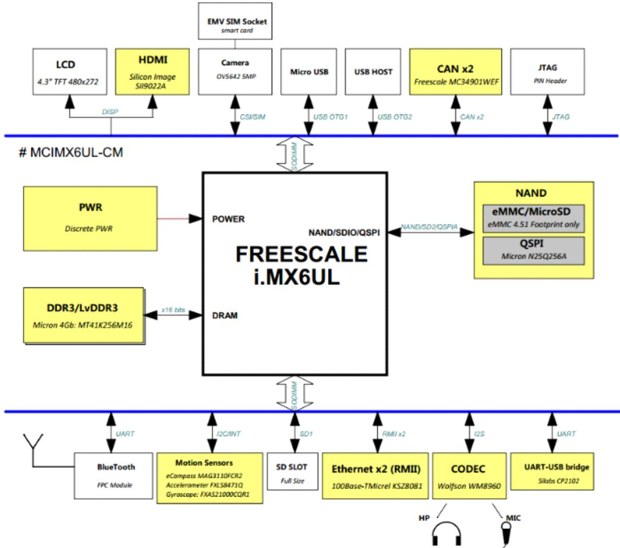
Figure 1. Block diagram
