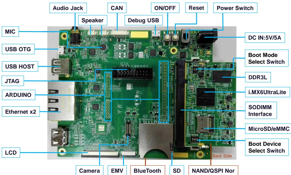
Figure 2. Overview of the i.MX 6UltraLite EVK board
