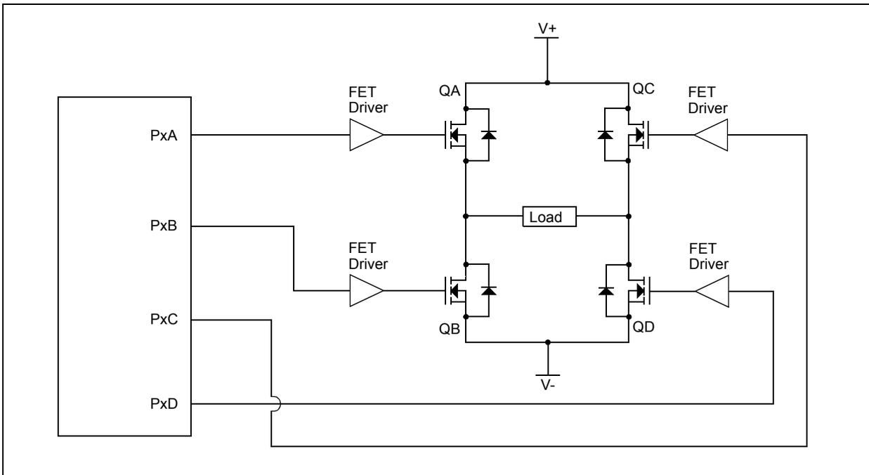
**FIGURE 23-11: EXAMPLE OF FULL-BRIDGE PWM OUTPUT**
