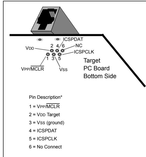
Another connector often found in use with the PICKit™ programmers is a standard 6-pin header with 0.1 inch spacing. Refer to [Figure 28-3](#).
