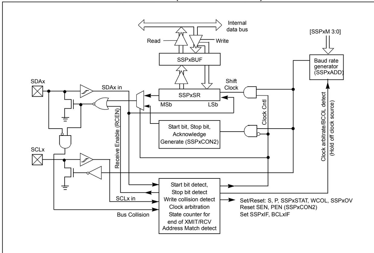
**FIGURE 24-3: MSSPx BLOCK DIAGRAM (I<sup>2</sup>C™ SLAVE MODE)**
