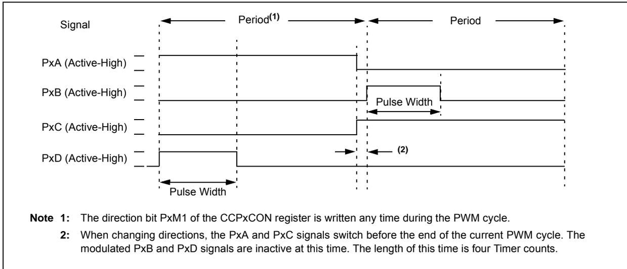
**FIGURE 23-13: EXAMPLE OF PWM DIRECTION CHANGE AT NEAR 100% DUTY CYCLE**
