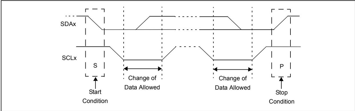
**FIGURE 24-13: I<sup>2</sup>C RESTART CONDITION**
