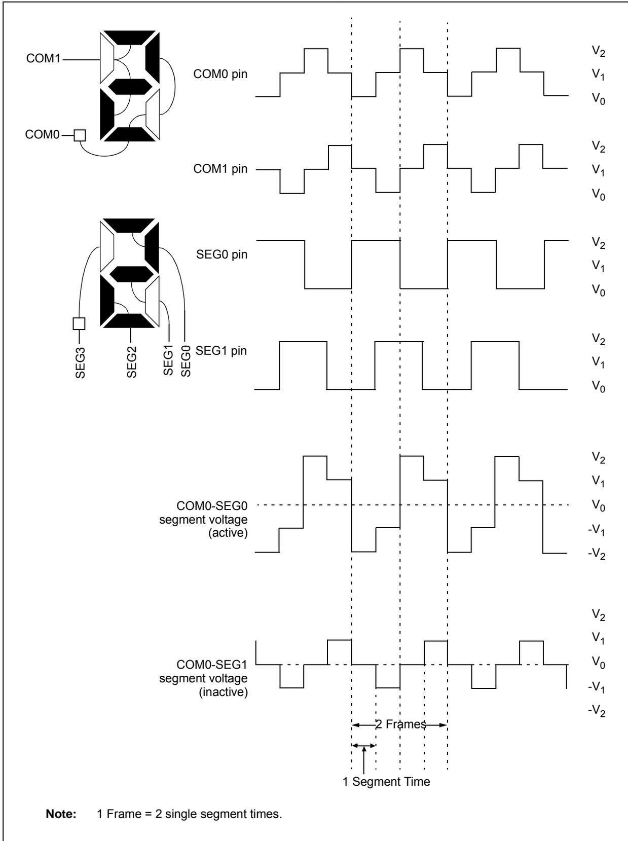
**FIGURE 27-11: TYPE-A WAVEFORMS IN 1/2 MUX, 1/3 BIAS DRIVE**
