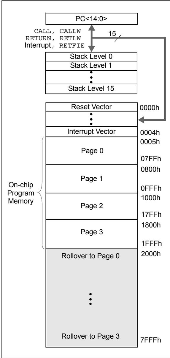
**FIGURE 3-2: PROGRAM MEMORY MAP AND STACK FOR PIC16F/LF1947**
