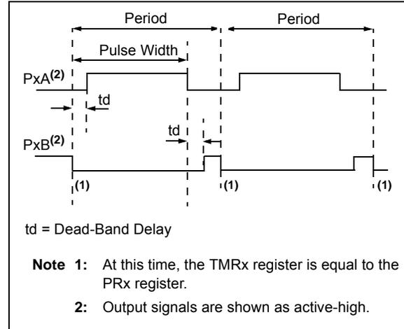
**FIGURE 23-17: EXAMPLE OF HALF-BRIDGE APPLICATIONS**
