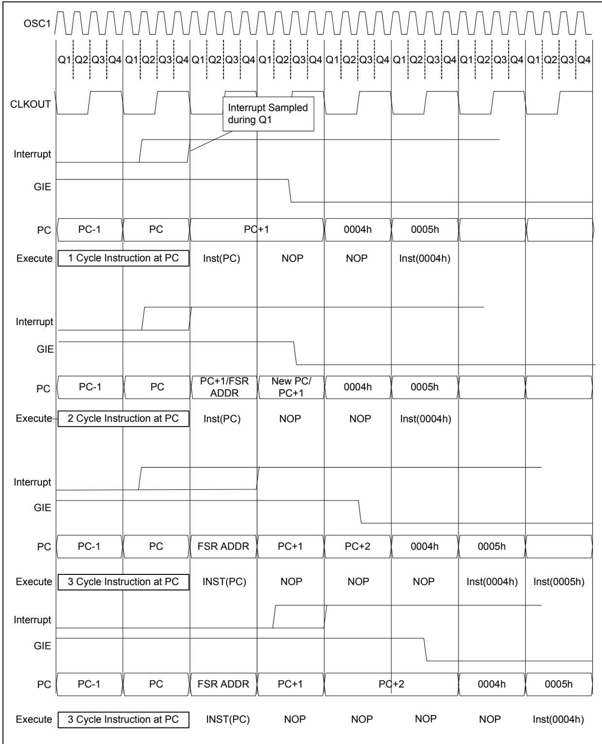
**FIGURE 7-4: INT PIN INTERRUPT TIMING**
