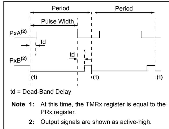
**FIGURE 23-9: EXAMPLE OF HALF-BRIDGE APPLICATIONS**
