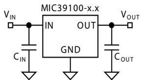
Figure 1. Capacitor Requirements
