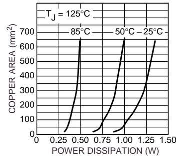
**Figure 3. Copper Area vs. Power-SO Power Dissipation ( $T_A$ )**
