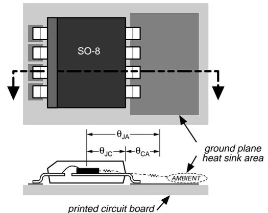
**Figure 1. Thermal Resistance**
