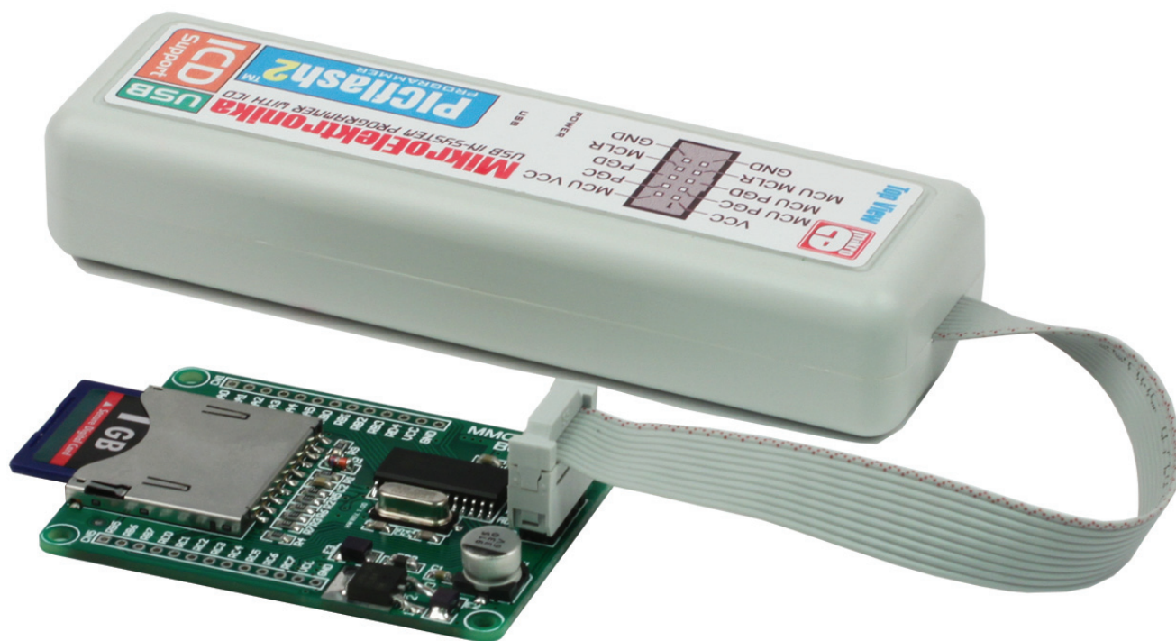
Figure 2: MMC Ready additional board connected to a programmer
