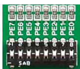
Figure 6-2: Tri-state DIP switch on PORTE
