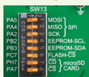
Figure 15-2: enabling microSD card commu- nication lines
