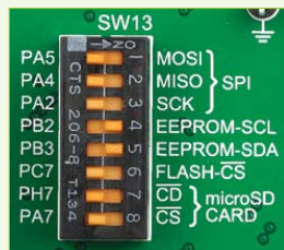
Figure 23-2: Activate SW13.4 and SW13.5 switches to enable pull-up resistors in I 2 C lines of Serial EEPROM.
