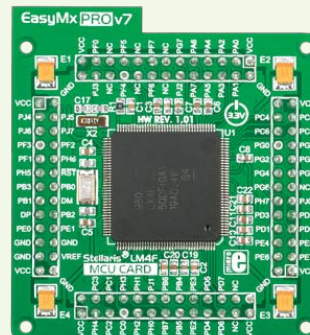
MCU card for Stellaris® LM4F series with LM4F232H5QD
