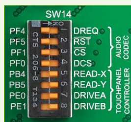
Figure 17-2: Turn on switches 5 through 8 on SW14 to enable Touch panel controller
