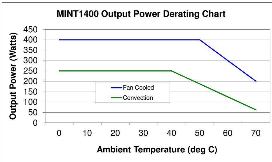
**Note:** For convection cooling, the power supply is required to be mounted on a heatsink or system chassis with a minimum of 150 in<sup>2</sup> of surface area.
