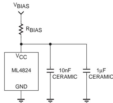
Figure 3. External Component Connections to V<sub>CC</sub>
