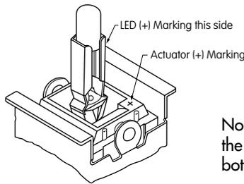
Note: When changing LEDs, match the positive polarity markings on both lamp base and actuator block.
