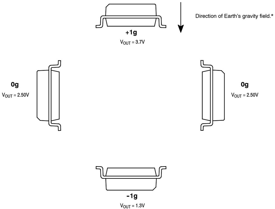
\* When positioned as shown, the Earth's gravity will result in a positive 1g output
