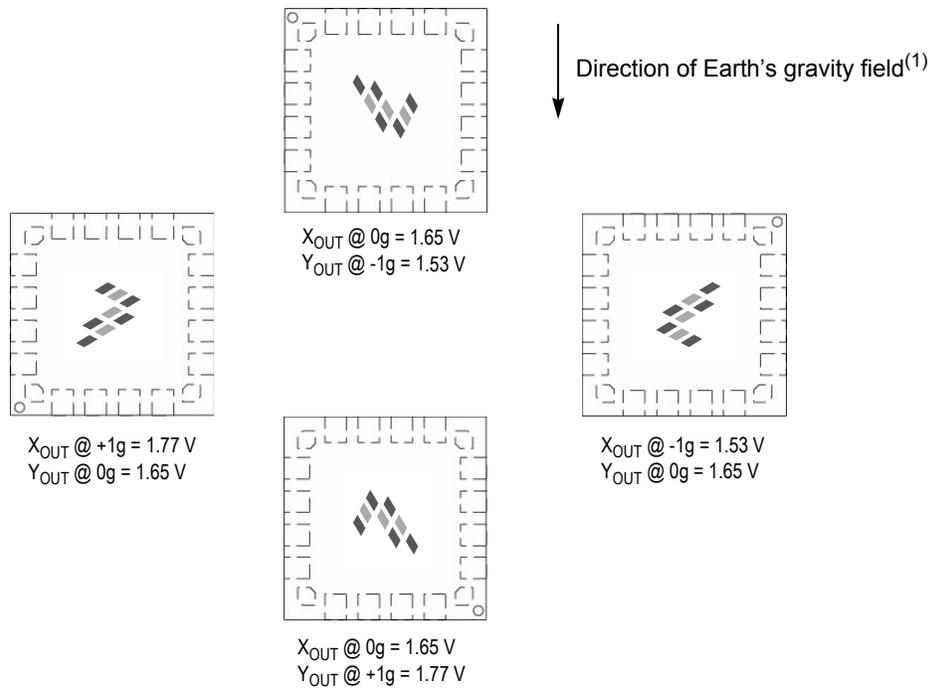
1. When positioned as shown, the Earth's gravity will result in a positive 1g output.
