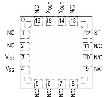
**Figure 1. Pin Connections**
