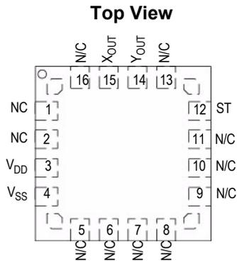
**Figure 4. Pinout Description**
