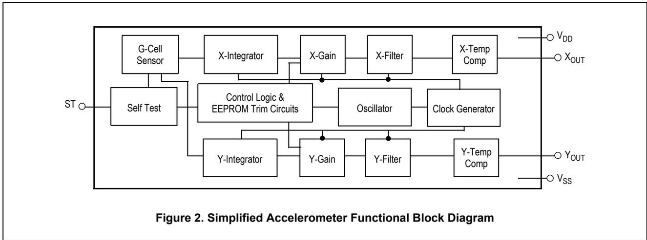
**Figure 2. Simplified Accelerometer Functional Block Diagram**
